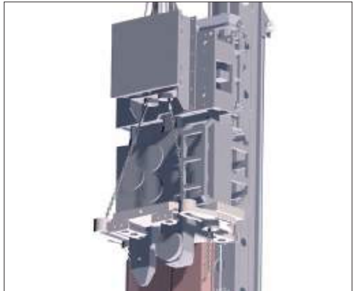
Double clamp and hydraulic sheet pile feeder
